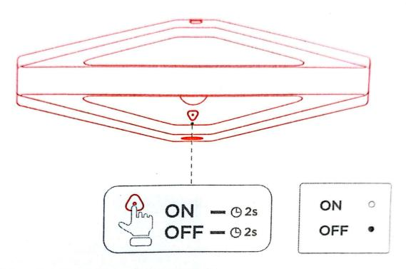
Press and hold the Power button for 2 seconds to power on.
