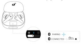
Once connected successfully, the earbuds will automatically reconnect to your device every time you slide open the charging case, as long as you haven't deleted the pairing history from your device.
