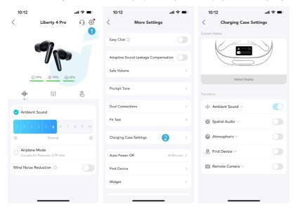
In the soundcore app, you can determine the functions you wish to appear on the charging case menu. There are a total of five functions available for smart control via the charging case:
