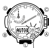
Auto light switch on indicator
