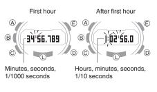
2. Press (E) to reset the elapsed time to all zeros.
