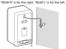
Prepare screws (not supplied) that are suitable for the wall material and strength. As a plasterboard wall is especially fragile, attach the screws securely in the wall beam. Mount the speakers onto a reinforced wall making sure that the heights of the right and left speakers are equal.
