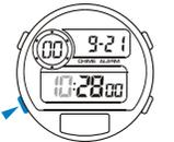
4. Press "D" to increase the number, press and hold to change at high speed;
