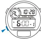
4. Press "D" to increase the minutes, press and hold to increase at high speed;
