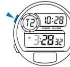
2. Press "D" to increase the hour, press and hold to increase at high speed;
